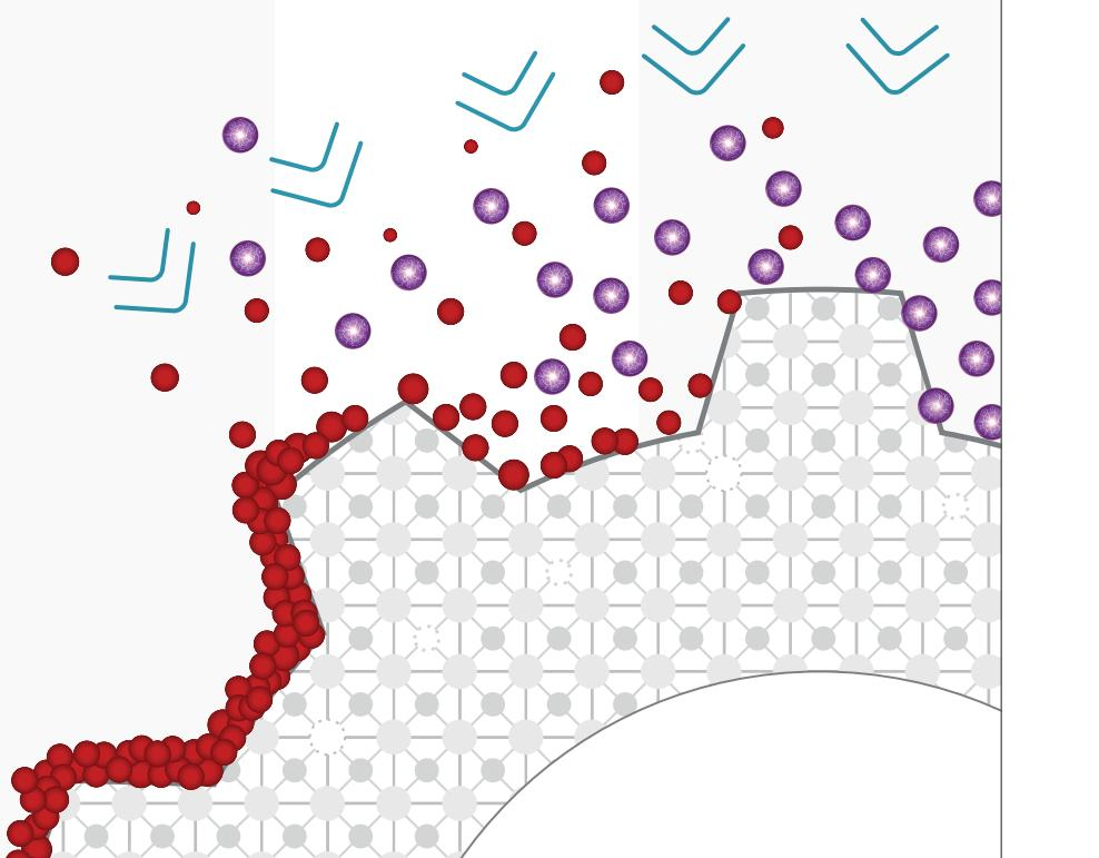
As noted earlier, a natural part of the plasma nitriding process is the ion bombardment known as sputtering, which actively **cleans the surface of components** before nitrogen diffusion begins.
