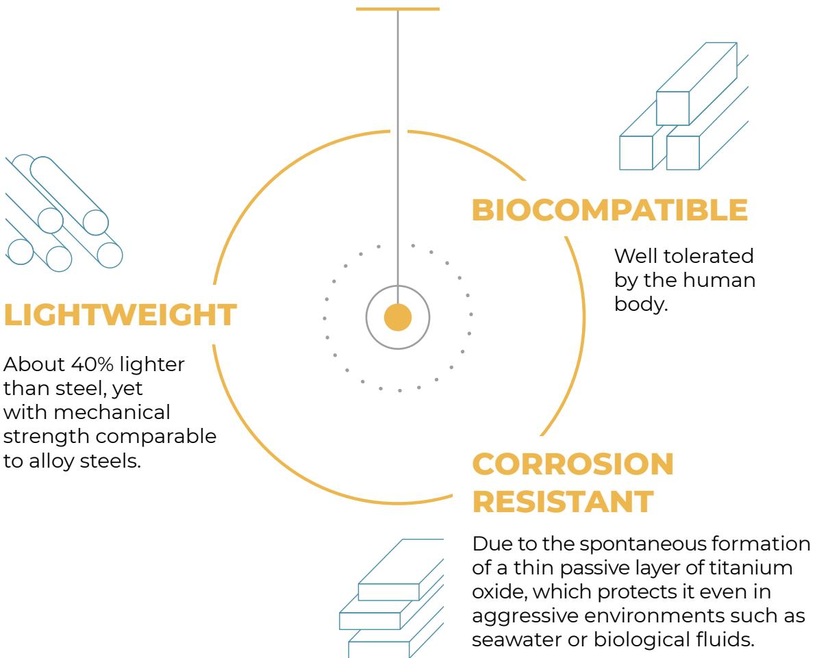
Despite its exceptional properties, titanium is **not widely used as a bulk metal** because extraction and refining are costly.
